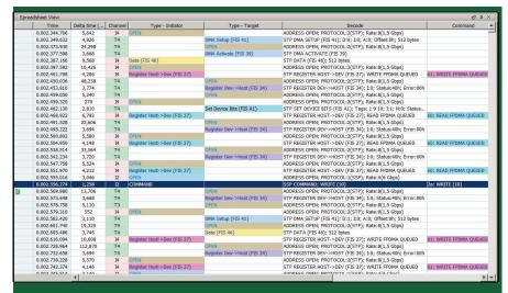
**Spreadsheet View** provides extensive decoding of frames, primitives, and Out-of-Band events, and sorts them to show the order they occured in. The displayed columns are chosen from an extensive list of fields and events.
