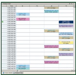
**Protocol View** shows the precise timing relationship of each D-Word in the trace. Useful for tracking the handshaking between products under test.
