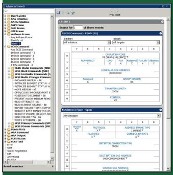
**Advanced Search** provides a way to search for sequences of events, either within a frame, or across multiple frames or events. It is identical to the Trigger Sequencer in appearance.
