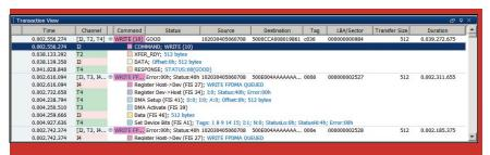
**Transaction View** shows each command in the order it was initiated. Commands may be expanded to show the frames associated with them, or collapsed so that only a summary of the command is shown.
