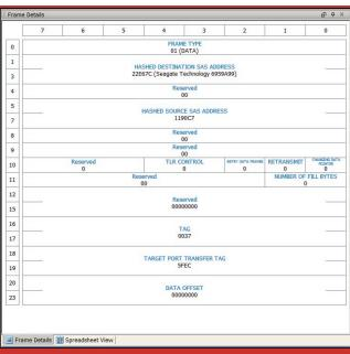
**Frame Details** shows each frame in the format used by the SAS or SATA specification.
